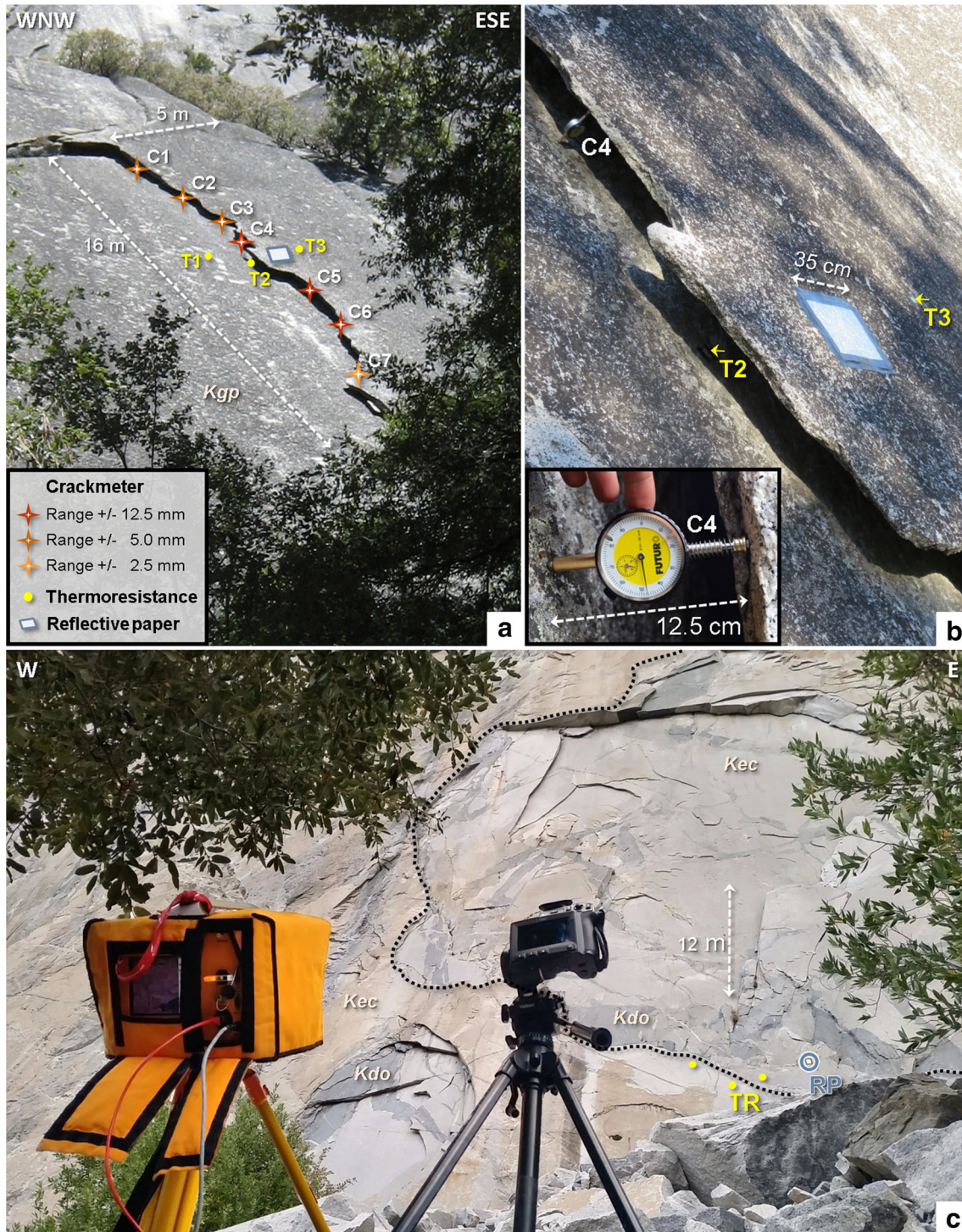
Fig. 2 Instrumentation setups at the Rhombus Wall flake and El Capitan. A Side view of the sub-vertical granodiorite exfoliation sheet at the Rhombus Wall flake (time shown is 13 Oct. 2015 at 12:05 PDT). The picture is taken from the position of both laser scanner and thermal camera. C#, crackmeter; T#, thermoresistance sensors; Kgp, Glacier Point granodiorite. Red, brown, and orange stars correspond to large, medium, and small size crackmeters, respectively. B Detail view of the area where the reflective paper was fixed on the Rhombus Wall flake (time shown is 13 Oct. 2015 at 16:55 PDT). The shadow on the rock is due to the vegetation surrounding the study site. C Front view of the granitic exfoliating rock wall monitored on El Capitan (time shown is 19 Oct. 2015 at 17:33 PDT). The black dashed line indicates the western boundary of a rockfall scar from 3 October 1976. All overhanging sections correspond to granitic exfoliation sheets. The foreground shows the laser scanner (left) and infrared thermal camera (right). Kec, El Capitan granite; Kdo, dikes of the oceans; RP, reflective paper; TR, thermoresistance sensors
