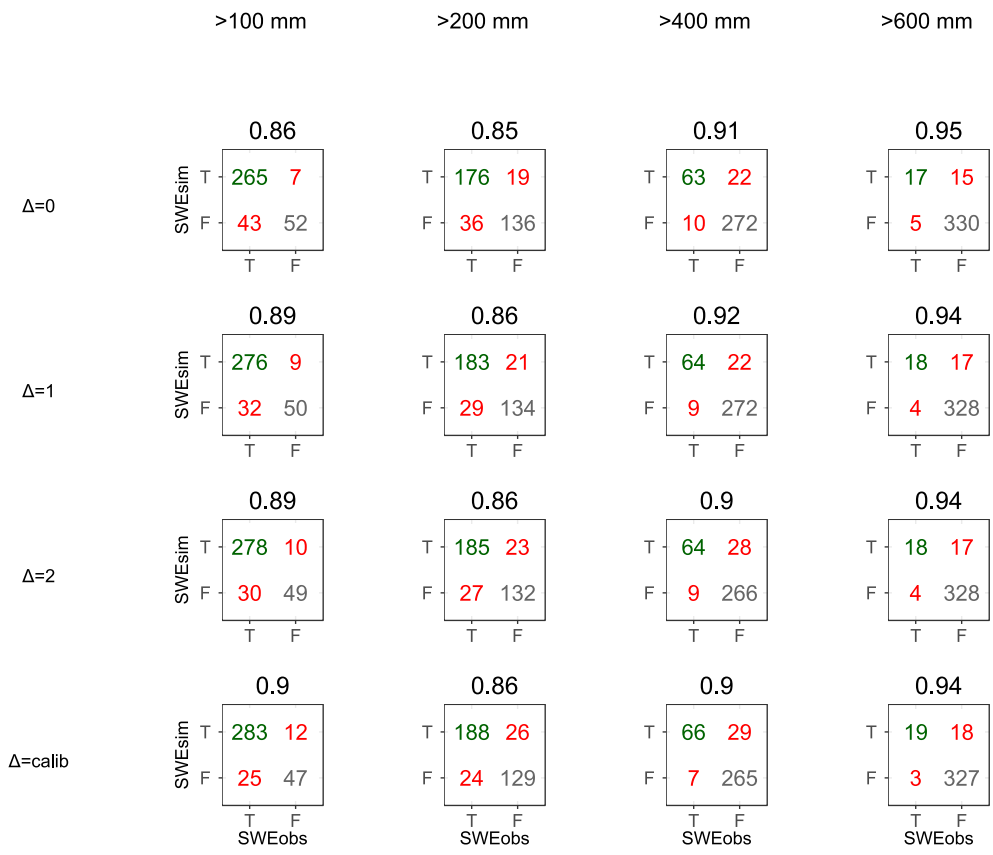
Figure D.9 – Confusion matrices and Overall Accuracy values obtained with the product QPE2-130 and the four variation interval configurations to reproduce the SWE quantity when applying SWE thresholds of 100, 200, 400 and 600 mm. T (TRUE) refers to threshold overrun (=Snow) whereas F (FALSE) indicates cases without threshold overrun (=NoSnow).
