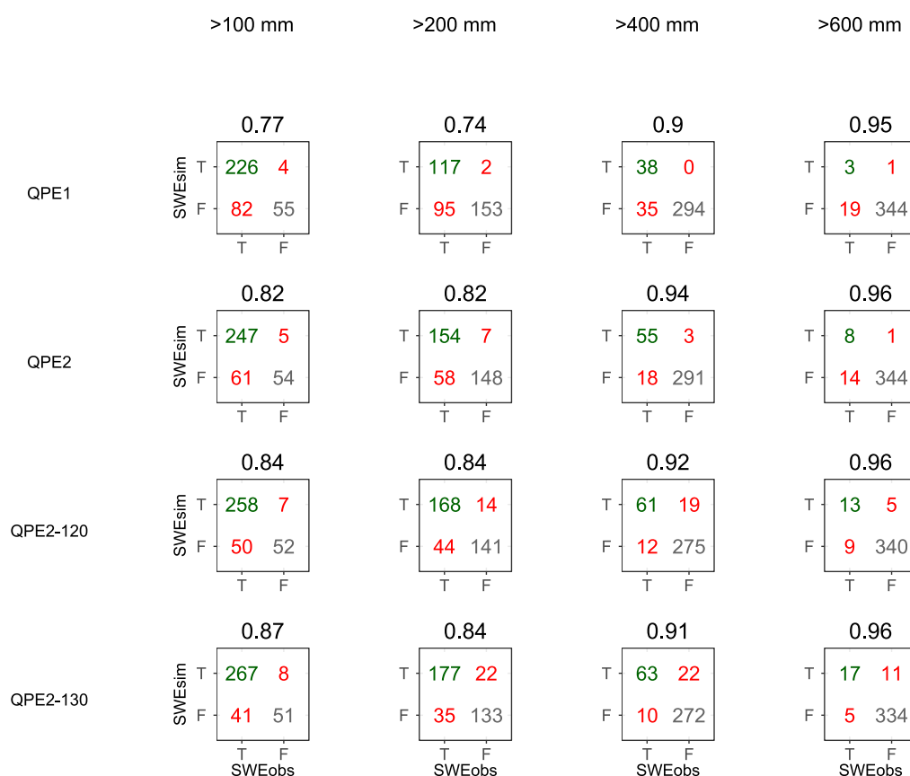
Figure 3.15 – Confusion matrices and Overall Accuracy values obtained with the four QPE products ( \Delta = 0 ) to reproduce the observed SWE values when applying SWE thresholds of 100, 200, 400 and 600 mm. T (TRUE) refers to threshold overrun (=Snow) whereas F (FALSE) indicates cases without threshold overrun (=NoSnow).
